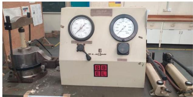
5. After the test is completed the cells have to be cleaned from the cells again, and the cells separated to prepare for next test. Done by using the 30 cm handle rod to mount the handle and pull out the inner circle.
