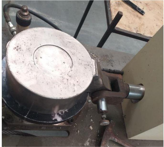
12. Finally when the component cells are completely coupled and secured with the clamp, connecting to the shear and axial pumps and the cells, apply slight load on the pump to tighten up connections.
